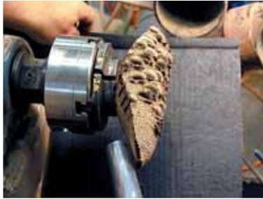
Step 7. After repositioning the work in his chuck, Dave checks that the "wings" on the pod are symmetrical by noting how far they extend along his tool rest.
