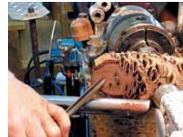
Step 3. Rough turn the bottom of the pod using a 1/2" bowl gouge. For a finishing cut, Dave prefers to use a pull-cut because he thinks that produces the cleanest cut. Do not use a scraper because it will tear the edges.
