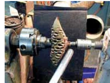
Step 4. Check that the tenon size will match your chuck. At this point, it may also be necessary to shift the live center placement to get a well-balanced foot on the pod. Note the gauge Dave uses to do this.
