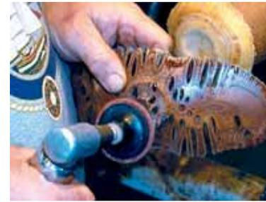
Step 18. A small sander with 80-grit abrasive is used to remove the nub left on the foot. Finer grits are then used to finish the foot area, and diluted shellac is again used as a sealer.
