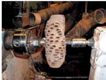
Step 2. Place the pod between centers on the lathe with the bottom towards the tailstock. Dave does not use a cone-shaped live center in order to minimize damage to the pod's foot.
