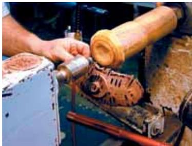
Step 14. Prepare to finish the foot by reversing the pod on the lathe. Dave uses a homemade support padded with leather to hold the work against the tailstock.
