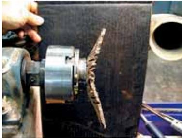
Step 10. Dave has finished turning the top side with the live center removed. Again use a sheet of blackened cardboard to check the form profile.
