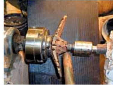
Step 9. The pod with the top rough turned about 1/4" thick. Keep the live center in place during all the roughing for better stability and safety.
