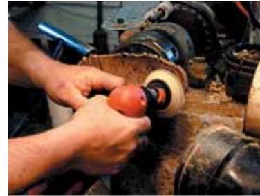
Step 12. Most mortals will need to start with a coarser grit, but Dave starts with 240. The lathe is off, and the sanding pad is positioned so its edge moves away from the pod.
