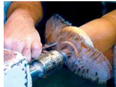
Step 15. This photo was taken using a flash while the work was turning. It shows Dave's well-controlled gouge making fine finishing cuts on the pod bottom side. Due to close quarters, Dave uses a 3/8" bowl gouge for these cuts.
