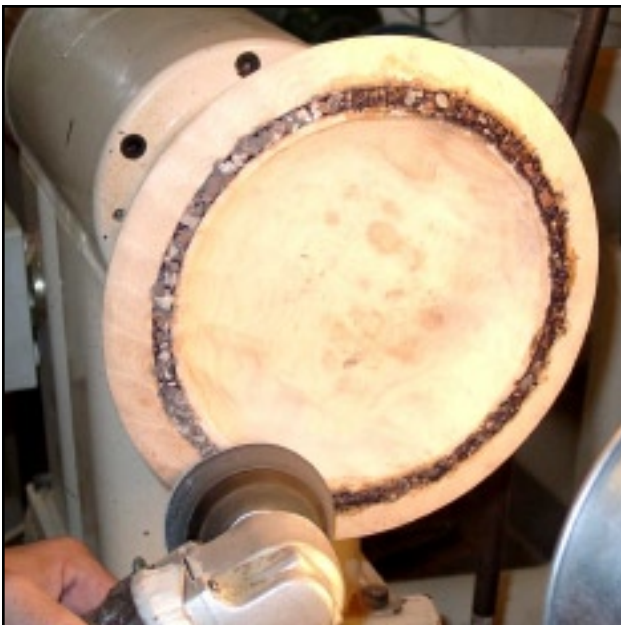
Use power sanding to finish the stone. Start with 60-80 grit and take the stone down until it's just flush with the wood surface.
