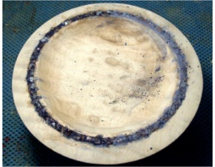
The stone glued-up with finer crushed material added around the coarser pieces. Tap the wood gently to settle the material then add superthin CA glue.
