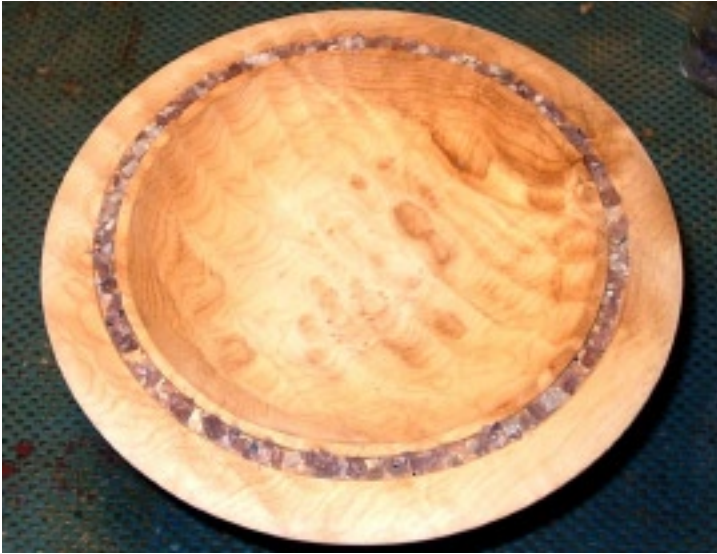
Coarse stone placed in the turned groove. It is often helpful to keep the wood in the lathe chuck and remove it from the lathe as a unit to maintain alignment.
