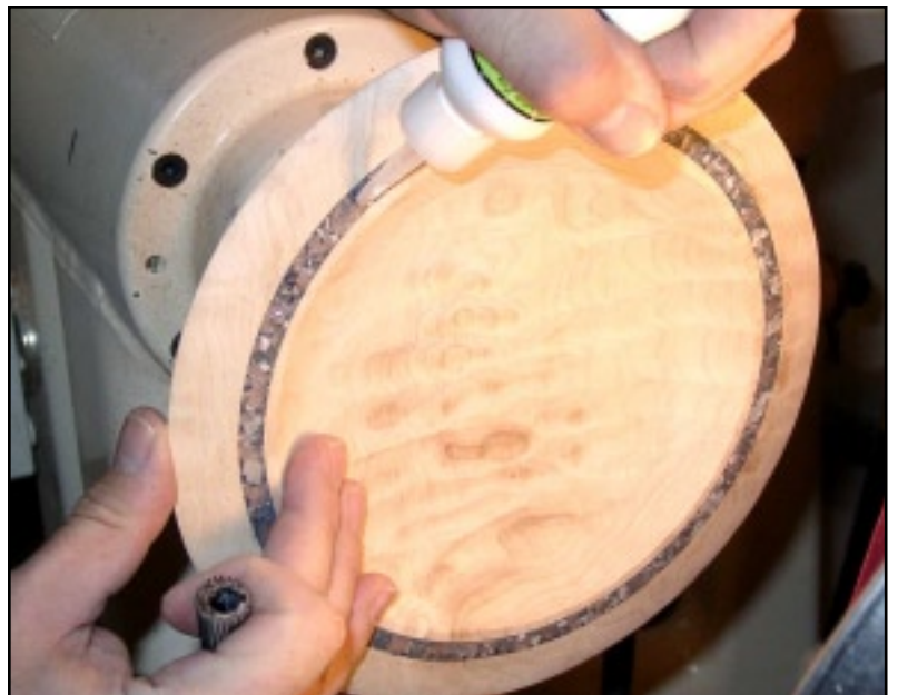
Progress through finer grits of sandpaper finishing the entire piece. If a large void occurs remove the wood plus chuck and repair, otherwise fill small voids with thick CA glue.
