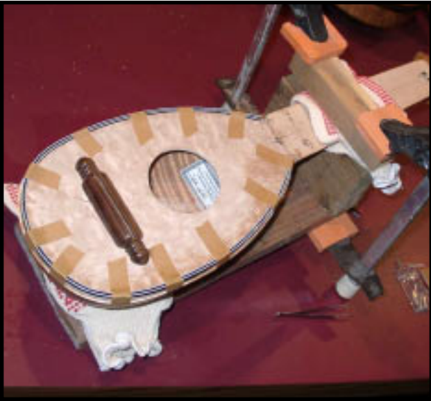
Inlaying paua shell, cellulose binding and guitar perfling into lute body (left), with inlay detail (right).
