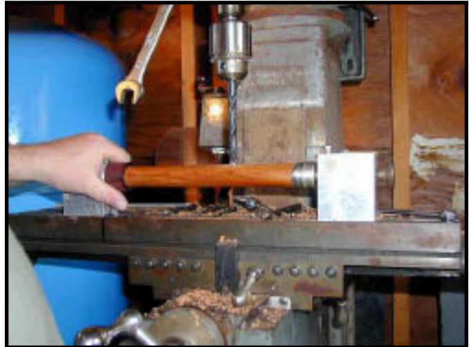
Drilling the flute sound holes.
