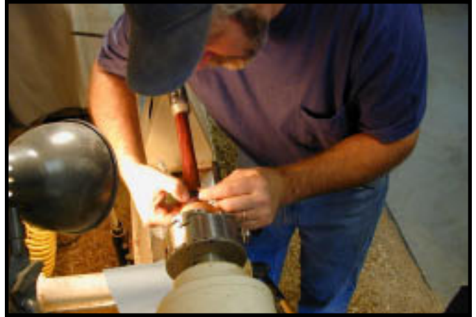
Adding paua shell inlay to the flute joints.
