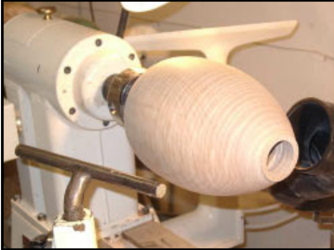
Turning lute body hollow form of fiddleback maple.
