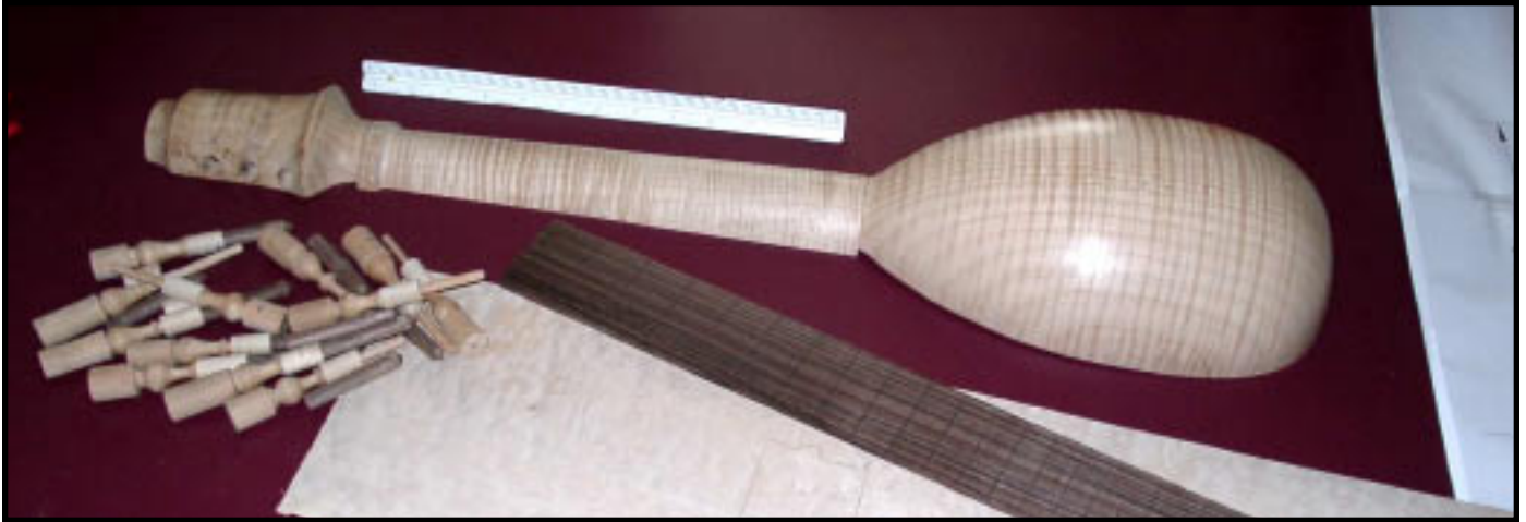
Lute head (curly maple), neck and body (fiddleback maple) and tuning pegs ready for final assembly.
