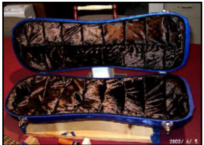
Handle, hardware, and crushed velvet lining added.
